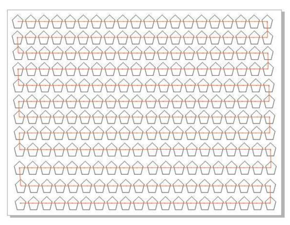
Here is the 'InsideBeforeOutside\_01' example after sequencing. The 'Shape Origin' location was used instead of 'Shape Center' for this example. Note that sequencing with Inside Before Outside selected is slower than without it.
