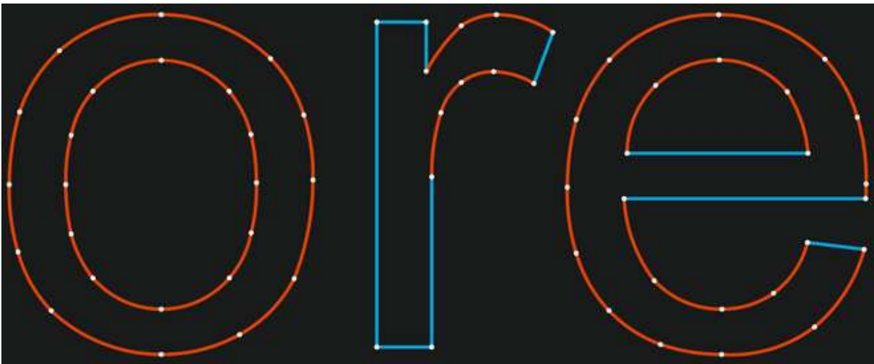
This is the same closeup as the CoreIDRAW DXF, but it shows the small number of segments and the smooth arcs made by the DXFTool Standard Edition.
